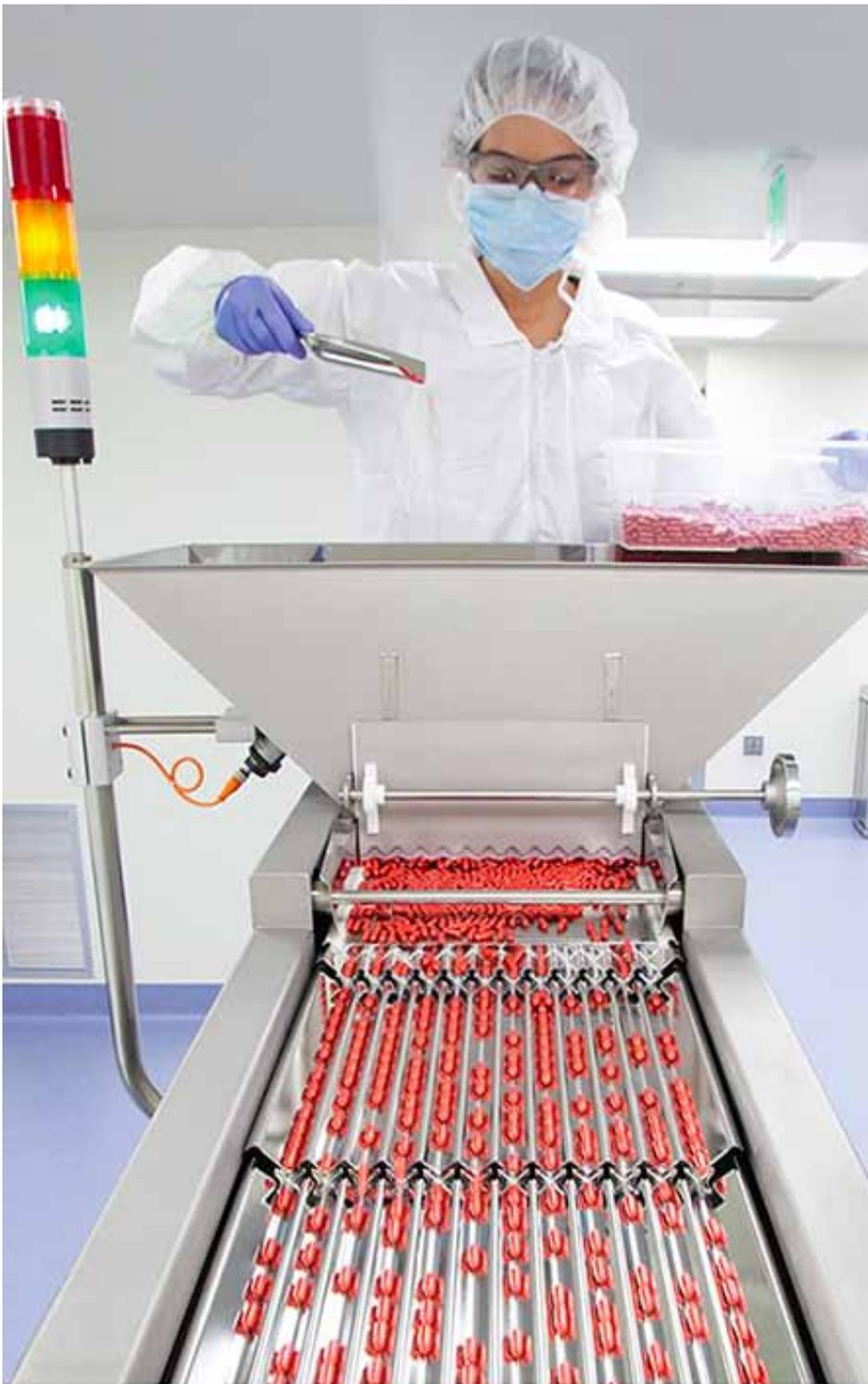
In Pharmatek's new packaging line, an operator is filling the hopper with capsules before entering the bottle filler.
